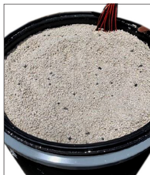
2 Loose Obexion FR poured over batteries
