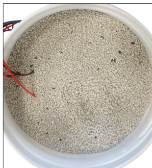
2 Loose Obexion FR poured over battery
