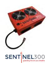
MODEL: Sentinel300 INPUT VOLTAGE DRAW: 12V or 24V DC 4A @ 12V or 2A @ 24V DC DIMENSIONS: 11.4" x 8.2" x 3.9" (29 x 20.8 x 9.9 cm) WEIGHT: 8lbs (3.63 kg) SOUND: 45dB AIR FLOW: 300 CFM
